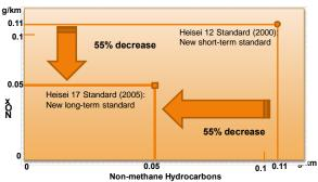
Emissions were measured by a new method (JE05) introduced with Heisei 17 emission gas standards
