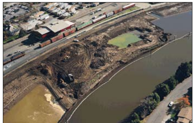
The Napa River in its most urban setting, in 2004. When floods hit, pools of industrial waste were washed across the city. Chemical companies have since cleaned up and converted these pits to flood terraces as part of the restoration work. Photo: Napa Flood and Water Conservation District
