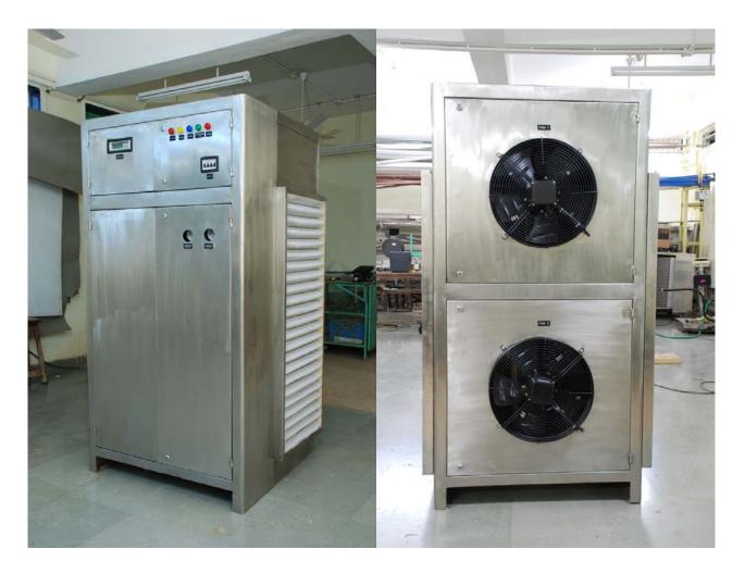
**Figure 4: Multi-Utility Air to Water Heat Pump, AW\_HP** *Currently Installed at an Automobile Manufacturing Unit*
