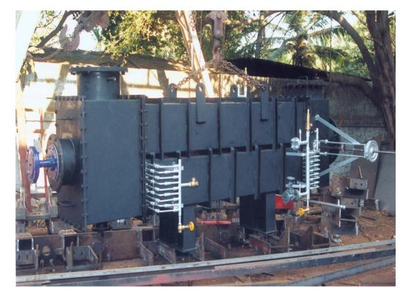
Figure 1: Matrix Heat Recovery Unit for Steam Generation for Installation on a 1250 kVA Genset
