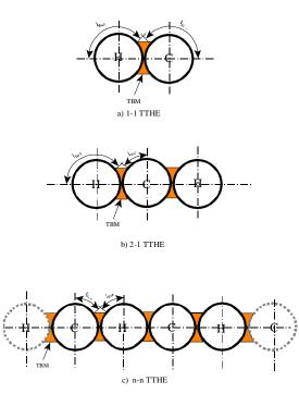
Figure 2: Sectional View of Three TT\_HE Configurations
