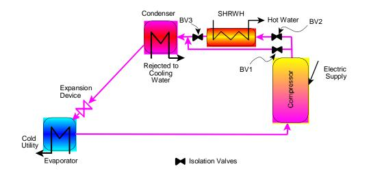
Figure 3: Refrigeration Circuit with Super Heat Recovery-Water Heater
