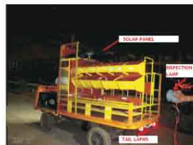
Mobile Work Station with Solar Panels, South East Central Railway.
