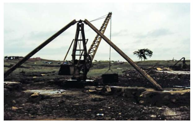
Collecting coal from the mine with the help of crane
