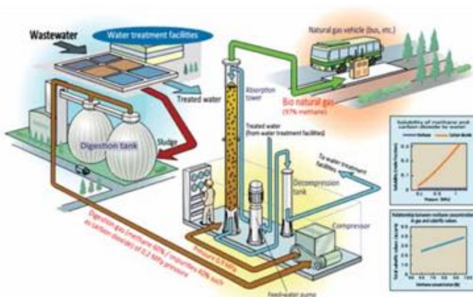
Figure 6: Schematic Diagram of the Biogas Generation System in Kobe City
