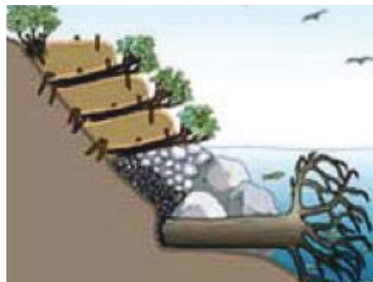
Figure 2.5: Cross-Section Illustration of Vegetated Revetments, Including Components Installed Below and Above the Water Line
