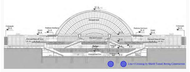
Figure 3.11: Tianjin West Railway Station Metro Line 4 Shield Tunnel Station Sectional Schematic Diagram
