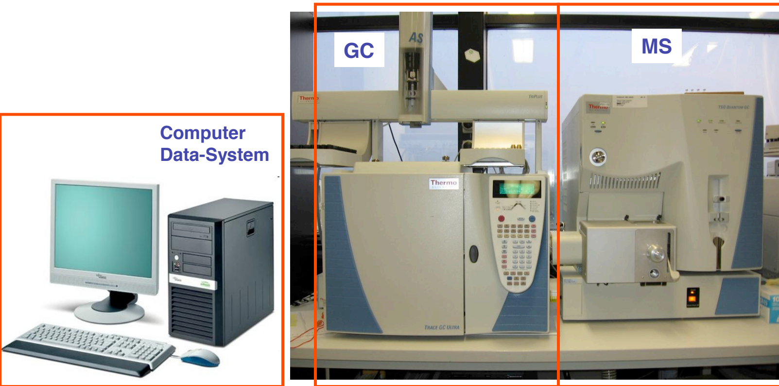
GC-MS-MS Quantum (Thermo Fisher Scientific) Gaschromatograph (GC) – Mass Analyser (MS)
